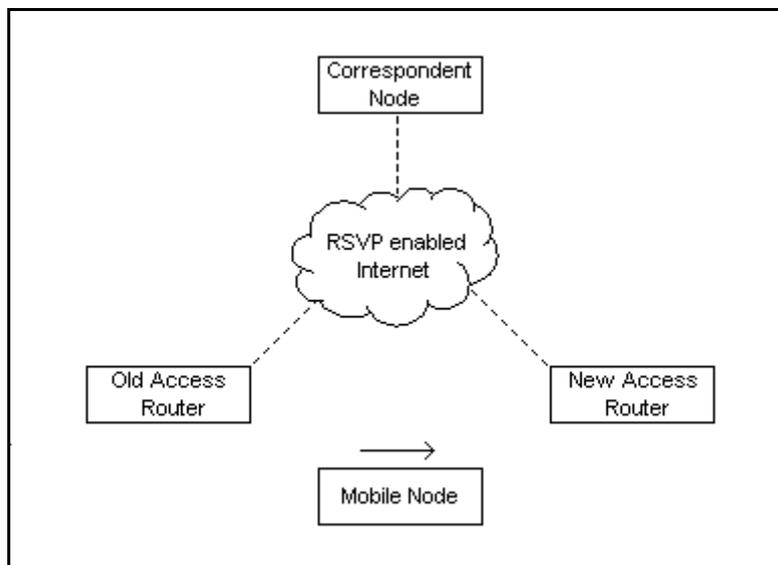
Figure 2. The network architecture that will be used to test the protocol. The mobile node is first connected to the old access router, and then the new access router. The two access routers may or may not be directly connected.
