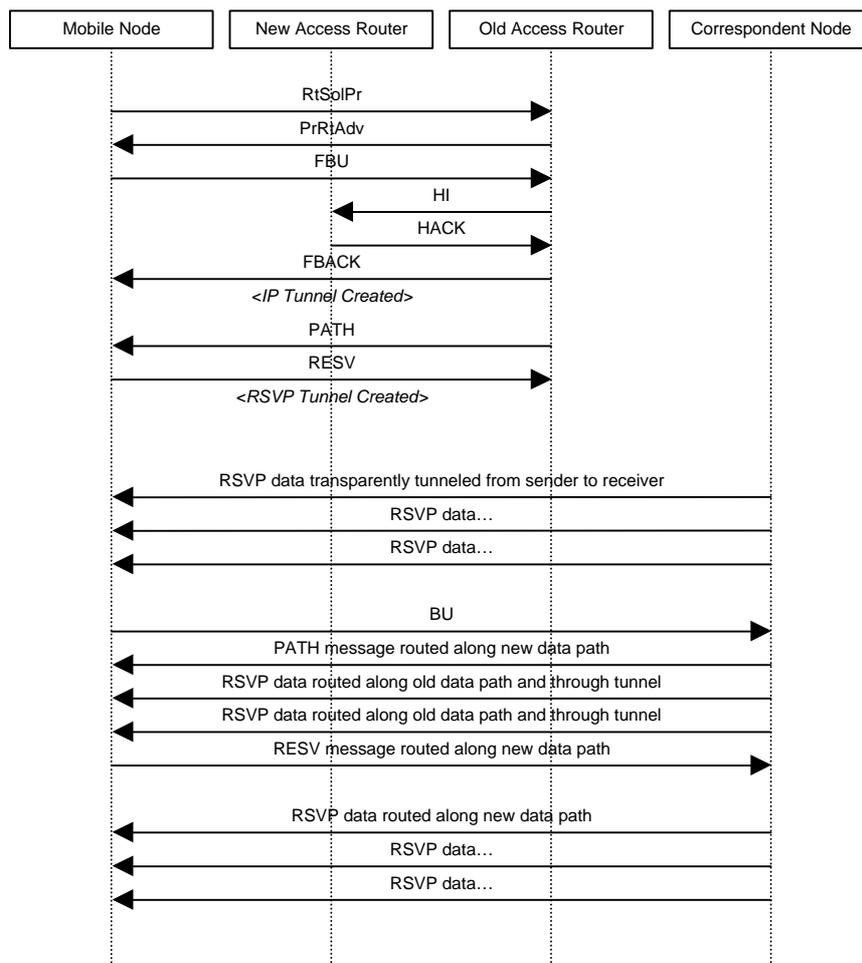
Figure 1. The protocol messages exchanged between the mobile node, old access router, new access router and correspondent node in the proposed protocol.
