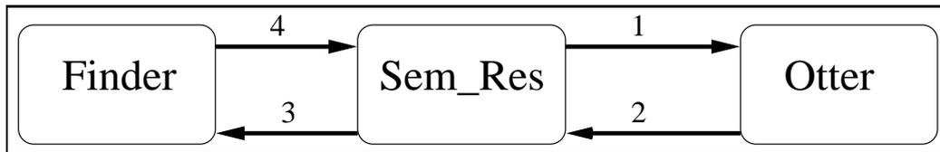
Figure 3: The flow of data in a single binary resolution inference step within the algorithm for semantic resolution.
