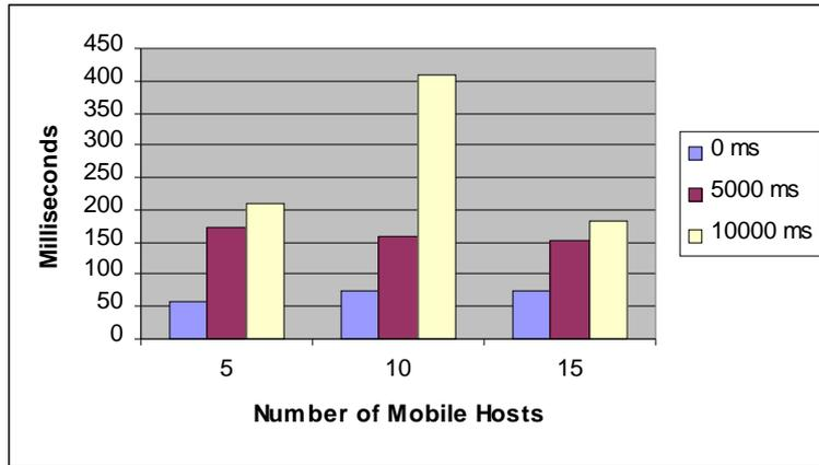
Figure 5. Transmission delay (packet arrival rate 500 ms).
