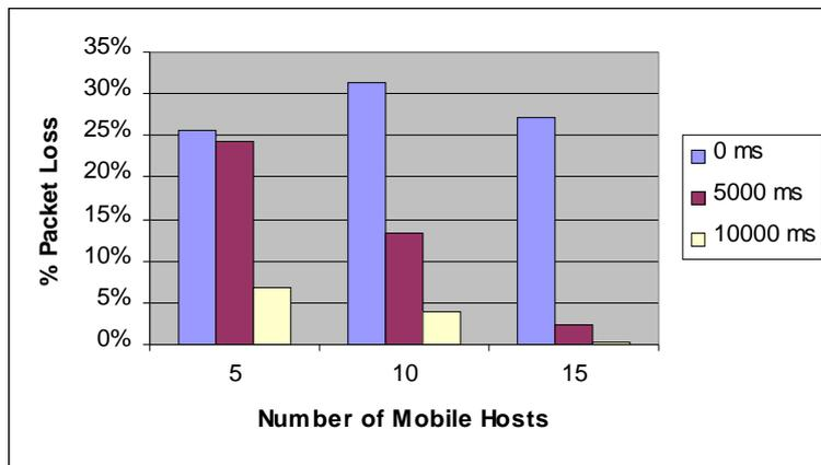
Figure 4. Packet loss (packet arrival rate 500 ms).
