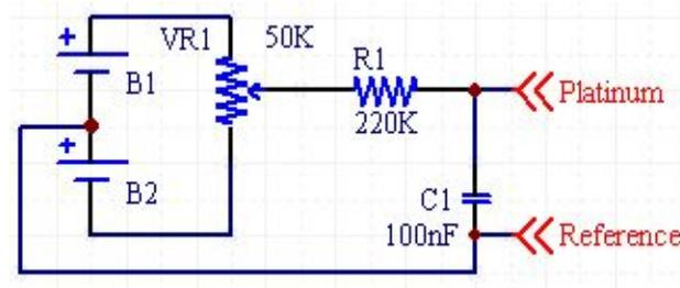
**Figure 1: Pt/Reference Electrode Simulation**
