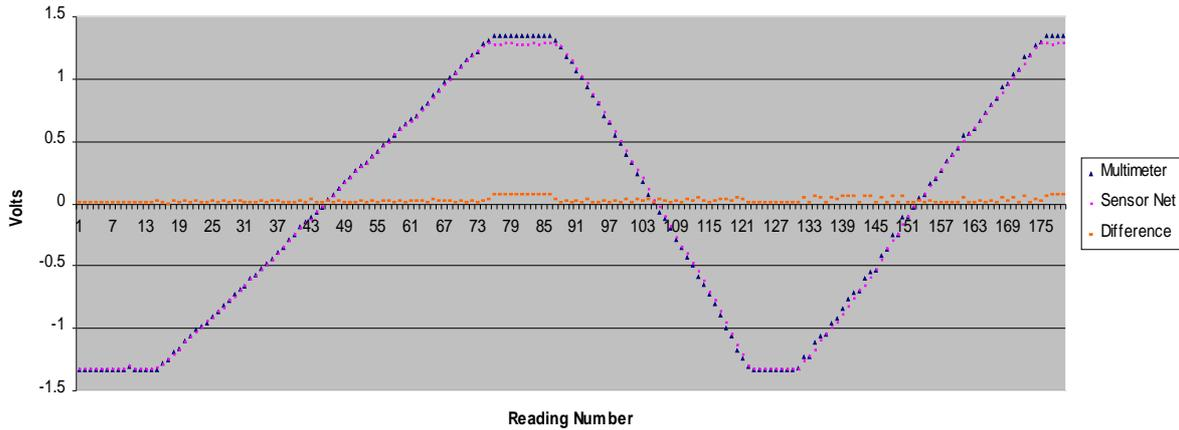
**Figure 2: Comparison of Actual and Measured Voltages**
